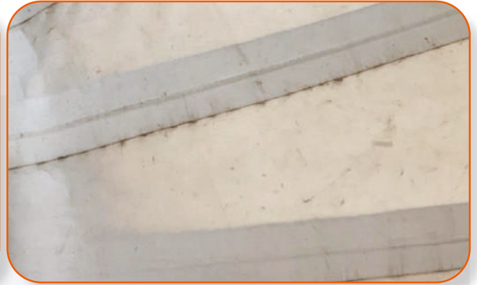
Normal Welding Bump Polyester Fabric Exposed
