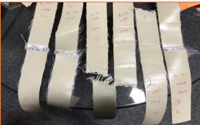
Weld Testing – Cold Peeled
