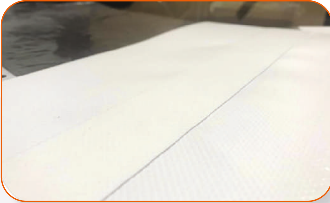
Normal Welding Bump Polyester Fabric Exposed
