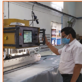
High Frequency Welding Machine (FORSSTROM, Sweden)
