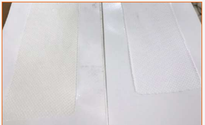
Weld Testing – Hot Peeled
